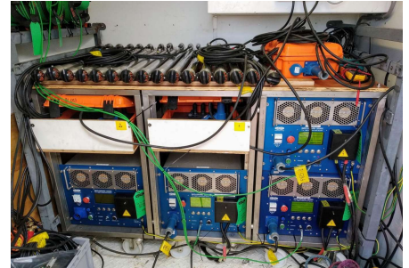
Pulsed Power Supplies at a 3D UHRS survey.
