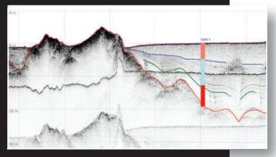
Bottom-track, filter and trace acoustic reflectors in the SonarWiz profile view.
